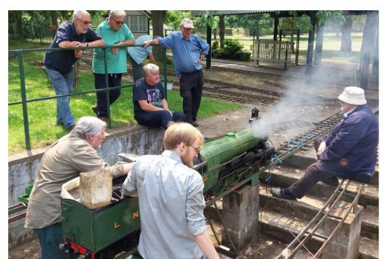
Here's the **A3** having a test steaming recently. The valve timing has now been corrected and there are just a few misc. leaks to be solved before it can have a steam test.
